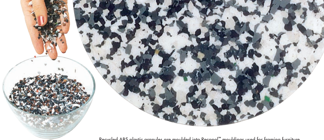
Recycled ABS plastic granules are moulded into Recopol™ mouldings used for framing furniture.
